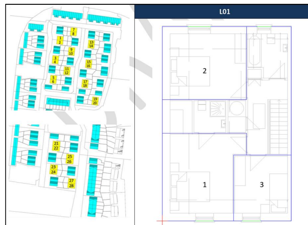
Figure 26: First Floor Plan House Type K1. IES first assessment highlighted house types that had rooms that failed to reach BER recommended standards
