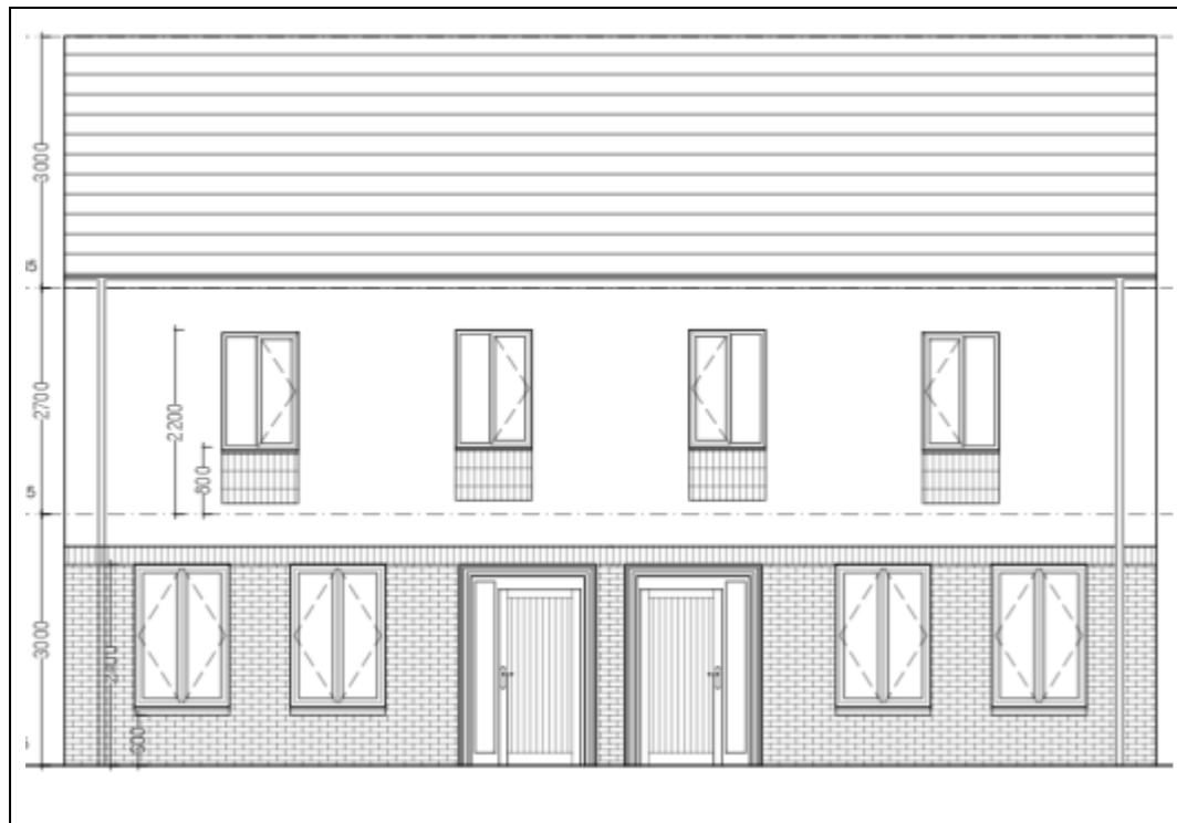
Figure 27: House Type K1 - bedrooms failed to reach BER recommended standards
