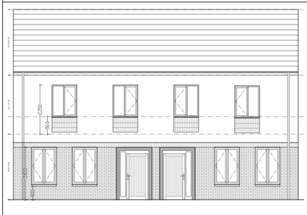
Figure 28: House Type K1 – First floor windows serving bedrooms have been increased in size
